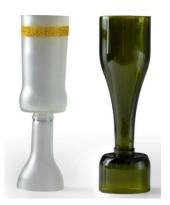
cloth to smoothen any rough spots and place the edge against the guide on the bottle cutter. (3) Adjust the bottle so that the glass cutter wheel is close to the bottom. You will end up with three pieces: the short bottom, the middle cylinder, and the top portion. Use the bottom and top for the goblet or candle holder, and the middle cylinder can be saved for interesting future projects.
