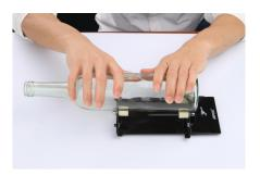
(2) Rotate the bottle toward one direction with two hands. Keep it firmly against the backstop and keep it moving while you're making the etching.
