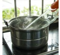
(2) Then put the bottle into cold tap water and rotate it. Repeat the above steps 2-3 times or more. When you repeat the steps, you may hear audible "clicks" indicating that the intact portions along the etching are now cracking. (Note: DO NOT use excessive force. Let the glass break itself.)
